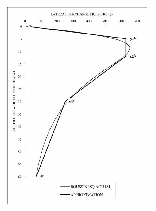
ANALYZE SHORING WALL USING BEAM ANALYSIS SOFTWARE TO DETERMINE DEPTH OF EMBEDMENT REQUIRED FOR STABILITY (I.E., BALANCE MOMENTS DUE TO LOADS ACTING BELOW THE LOWEST BRACING LEVEL).
