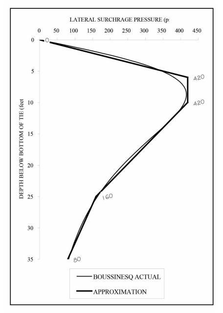
ANALYZE SHORING WALL USING BEAM ANALYSIS SOFTWARE TO DETERMINE DEPTH OF EMBEDMENT REQUIRED FOR STABILITY (I.E., SUM OF MOMENTS ABOUT BRACING LEVEL EQUAL TO ZERO).
