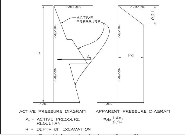
Figure 4-1: Construction of an Apparent Pressure Diagram
